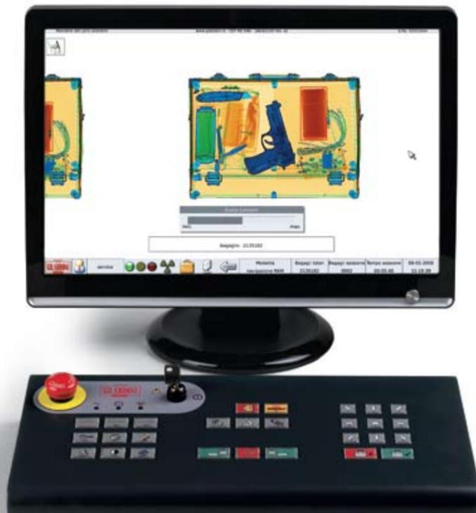
Operator console with widescreen LCD monitor
