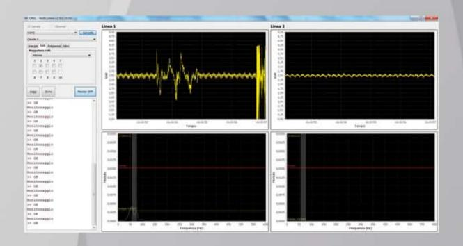
The NUS unit is supplied with a management software with which you can set the various configuration parameters. The software also has a graphical interface that allows real-time display of both the acquired and processed signals. The software can communicate with the central system locally through its USB connection, or remotely via LAN connection with TCP / IP protocol.
