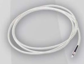
Fiber Multimode 62,5 / 125 of small diameter, high flexibility, ideal for cable distribution systems with terminal connection. Attenuation at 850 nm of 0.35 dB / km Bandwidth at 850 nm equal to 160: 300 MHz for Km Operating temperature: - 25 ° / 80 ° C.
