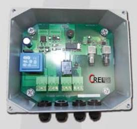
The unit FOS is constituted by an electronic type STANDALONE, compact and user-friendly, where inside there is a microcontroller. The module, which has the function of emitting a light beam modulated, transmitted over an optical fiber, and to analyze the same signal. If the signal transmitted by the control unit is interrupted, or does not match the one sent, the controller enters in alarm State.
